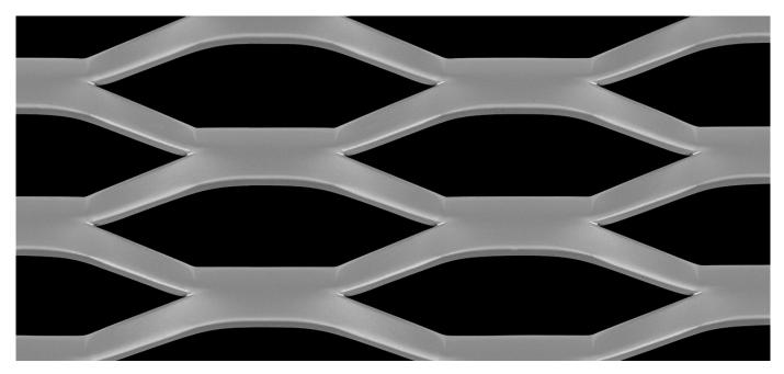
LW Pitch:121.92mmStrand Width:10.00mmSW Pitch:34.00mmThickness:3.00mmWeight:4.76 kg / m2Open Area:41%
